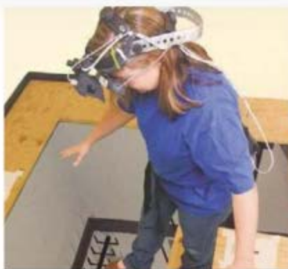
In 2007 a Georgia Tech team began researching what visual elements of an AR experience are needed to trigger realistic physiological and behavioral responses in users. This AR testbed presented the user with a scary virtual "pit" in the floor of an otherwise normal physical room. Ten years later the team built an updated version of the pit to explore how advancements in computer graphics have affected the users' experience.
